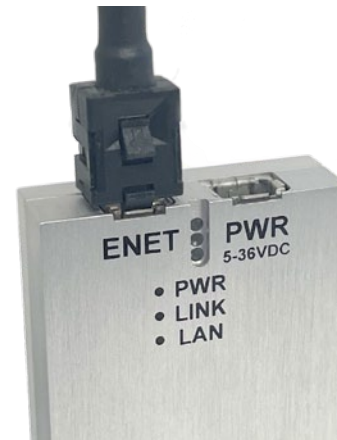
FIGURE 2-3: POWER & ETHERNET CONNECTIONS
