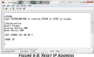
FIGURE 0-0: RESET IP ADDRESS
