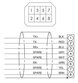
FIGURE 4-6: 100BASE-T ETHERNET PIN-OUT
