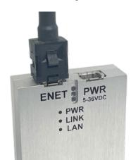
FIGURE 2-3: POWER & ETHERNET CONNECTIONS
