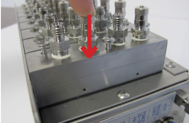
FIGURE 6.5: SENSOR PACK INSTALL
