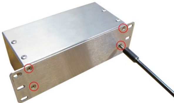
FIGURE 6.11: REMOVE BOTTOM MOUNTING PLATE
