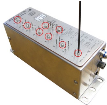
FIGURE 6.12: REMOVE TOP PLATE
