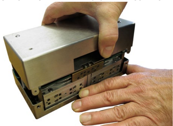
FIGURE 6.14: SEPARATE THE CASE HALVE SCREWS
