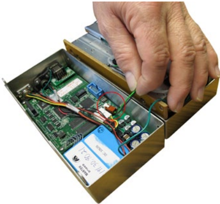
FIGURE 6.16: DISCONNECT THE QUICK ZERO SOLENOID
