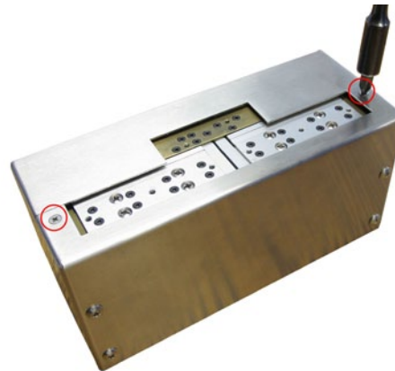
FIGURE 6.13: REMOVE THE CASE HALVE SCREWS
