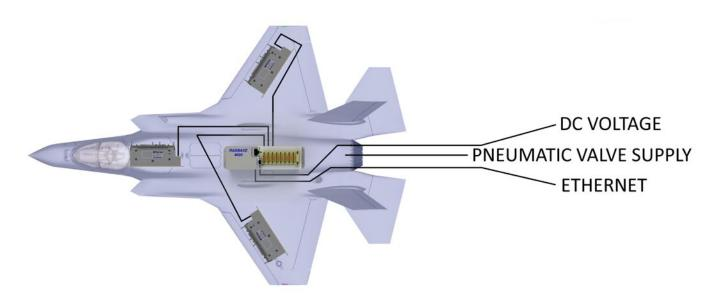
Shown using ERAD4000 mounted in the test article. Alternate system configuration uses DSM4000 installed under the test section or in the control room.
