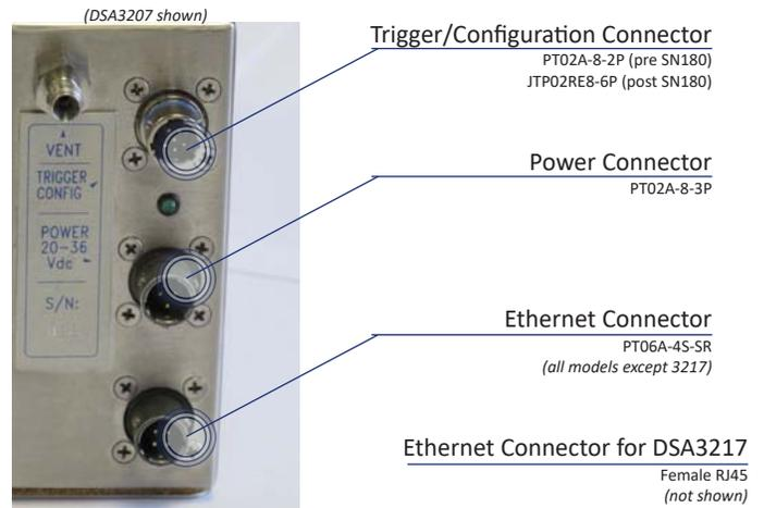
Note: DSA3000 series, and some DSA3200/3300 series were 10Base-2 and used a BNC connector of Ethernet connectivity. Standard 50ohm BNC cables can be used on these modules.
