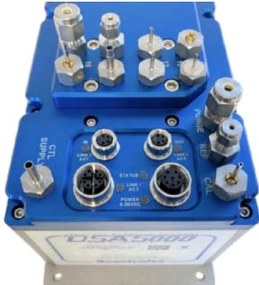
All pneumatic inputs use a 5/16"x24 female thread matching the SAE J1926-1\* standard. Scanivalve offers several fitting kits that can be installed on the modules when manufactured or different kits can be purchased. This provides flexibility to change out input fittings on a module-wide or channel-to-channel basis.
