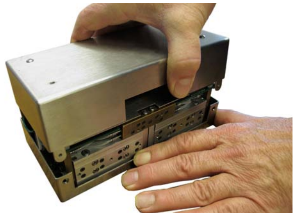
FIGURE 6.14: SEPARATE THE CASE HALVE SCREWS
