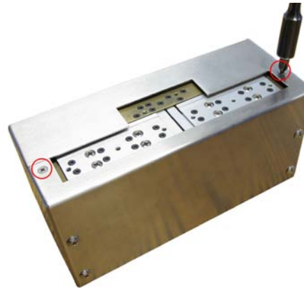
FIGURE 6.13: REMOVE THE CASE HALVE SCREWS
