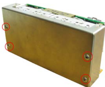
FIGURE 6.17: REMOVE THE CORE
