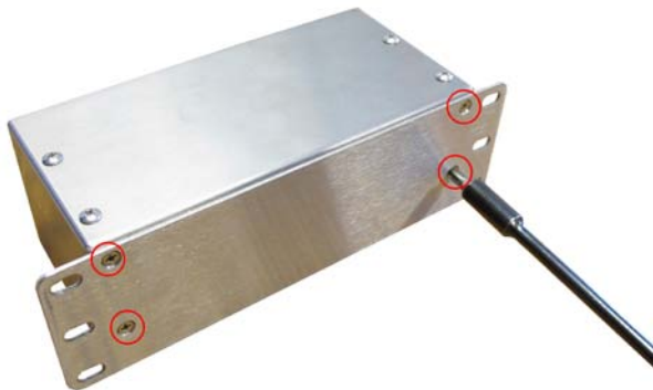
FIGURE 6.11: REMOVE BOTTOM MOUNTING PLATE
