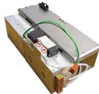
FIGURE 6.19: REMOVE THE MANIFOLD
