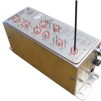
FIGURE 6.12: REMOVE TOP PLATE
