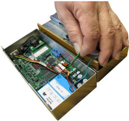
FIGURE 6.16: DISCONNECT THE QUICK ZERO SOLENOID
