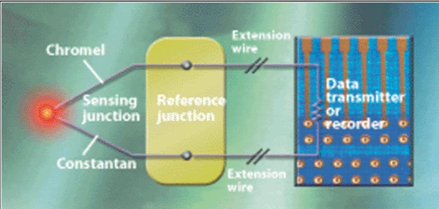
This temperature-measuring component consists of two dissimilar conductors—in this case, Chromel and constantan—welded together at their ends to form a junction. As heat applies to the junction, a voltage develops across it. This voltage is proportional to the temperature rise.
