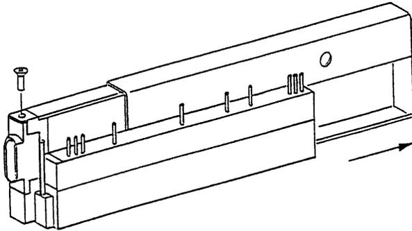
1. Remove the single screw holding the case in place and carefully slide the case off of the module.
