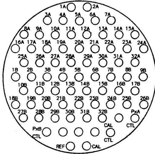
Figure 11 - ZOC22B TCU Pneumatic Connector
