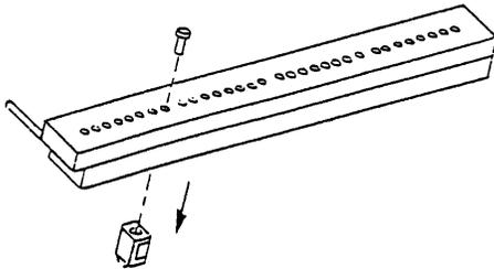
4. The sensors are held in place by screws that have been drilled through. Remove the failed sensor and replace it. Use the same screw.
