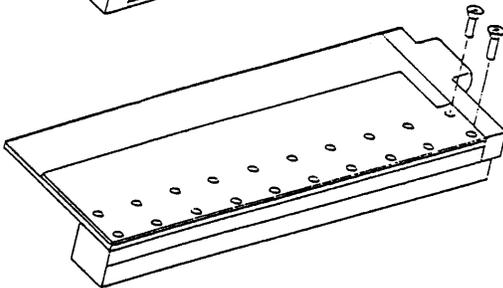
3. Turn the module over and remove the twenty(20) screws that hold the sensor housing in place. Be careful not to stress the circuit board during this step.
