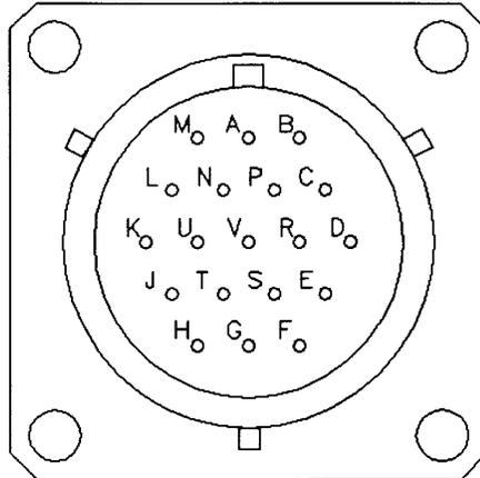
Figure 12 - ZOC22B TCU Electrical Connector
