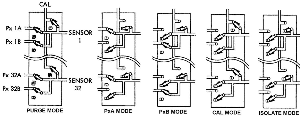
Figure 7 - ZOC22B/23B Valve Logic - X2 valve shown
