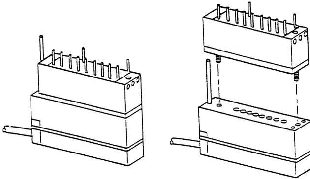
2. Remove the two(2) set screws, one at each end of the valve body and lift the valve body from the sensor pack.
