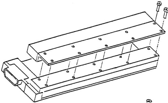
2. Remove the ten(10) screws holding the valve block in place and lift the valve block from the module body.
