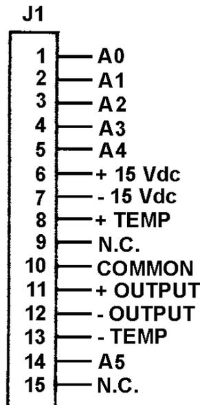
Figure 6 - ZOC22B/23B/Px Input/Output Connector
