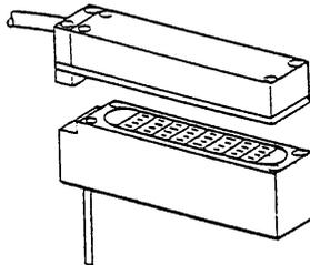
3. Remove the four(4) set screws from the sensor pack top cover and remove the cover.
