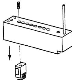
4. The sensors are held in place by special screws. Remove the screws and the failed sensor. Install the new sensor using the same or similar screw.
