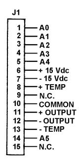
Figure 6 - ZOC22B/23B/Px Input/Output Connector
