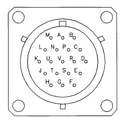
Figure 12 - ZOC22B TCU Electrical Connector
