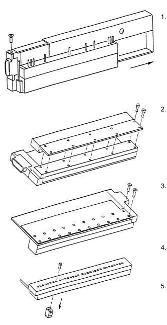
Remove the single screw holding the case in place and carefully slide the case off of the module.
