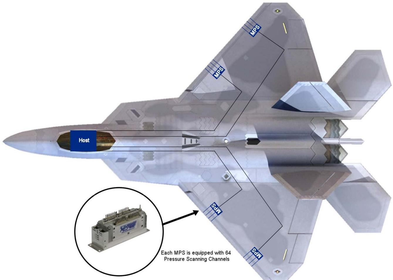
The MPS4264 is an intelligent 64 channel pressure measurement device. This device is a stand-alone scanner and handles all of the A/D conversion at the module level. Communication to the module is Ethernet TCP/IP or UDP. A TCU (Thermal Control Unit) is available to help stabilize sensor temperature in extreme conditions.
