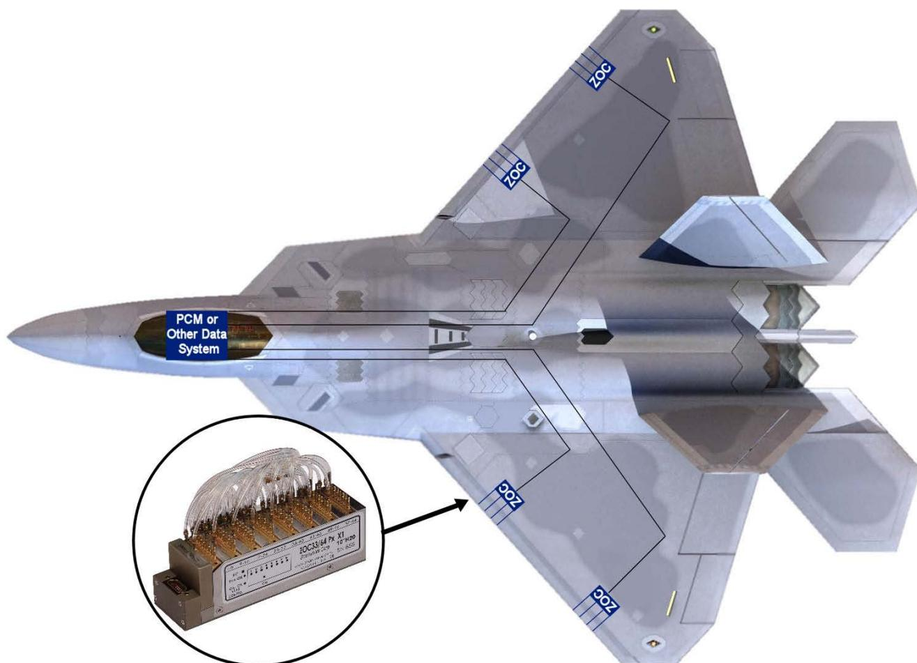
There are commercially available interface cards from flight test data system companies designed to work with Scanivalve products. ZOC scanners output an amplified analog signal which is then collected by the interface cards.
