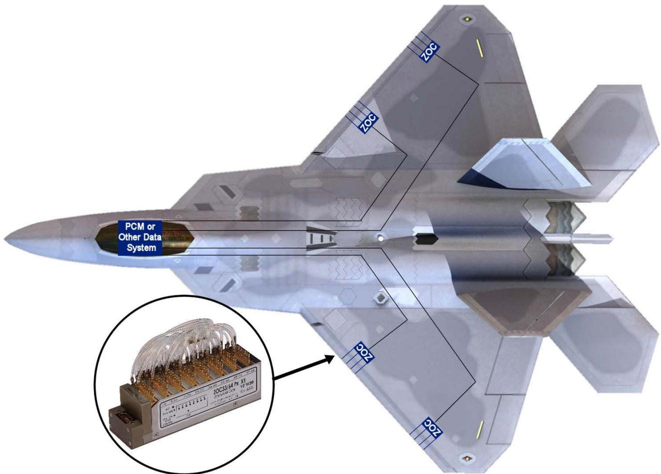
There are commercially available interface cards from flight test data system companies designed to work with Scanivalve products. ZOC scanners output an amplified analog signal which is then collected by the interface cards.
