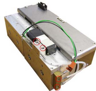
FIGURE 6.19: REMOVE THE MANIFOLD
