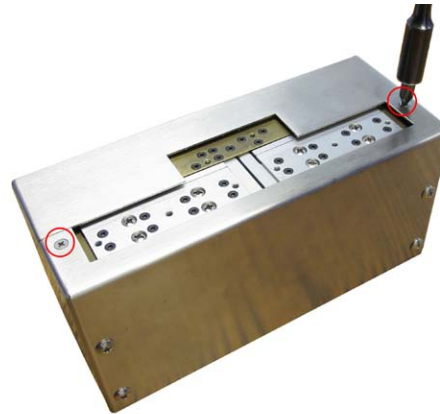
FIGURE 6.13: REMOVE THE CASE HALVE SCREWS
