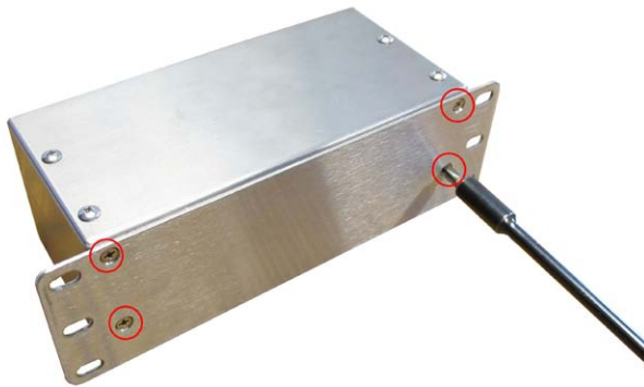
FIGURE 6.11: REMOVE BOTTOM MOUNTING PLATE
