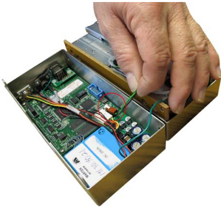
FIGURE 6.16: DISCONNECT THE QUICK ZERO SOLENOID
