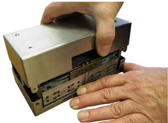
FIGURE 6.14: SEPARATE THE CASE HALVE SCREWS
