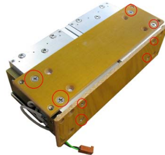
FIGURE 6.18: REMOVE THE INSULATORS
