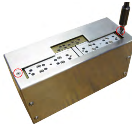
FIGURE 6.13: REMOVE THE CASE HALVE SCREWS
