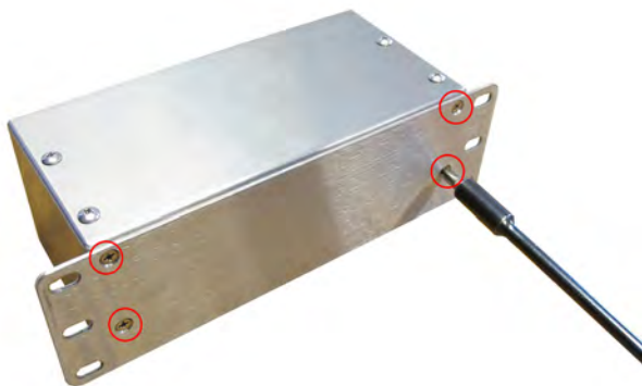
FIGURE 6.11: REMOVE BOTTOM MOUNTING PLATE
