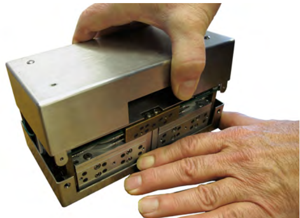
FIGURE 6.14: SEPARATE THE CASE HALVE SCREWS
