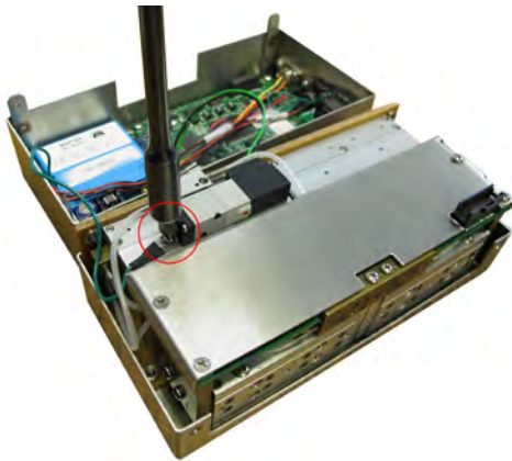
FIGURE 6.15: REMOVE THE GROUND WIRE
