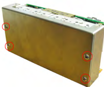
FIGURE 6.17: REMOVE THE CORE
