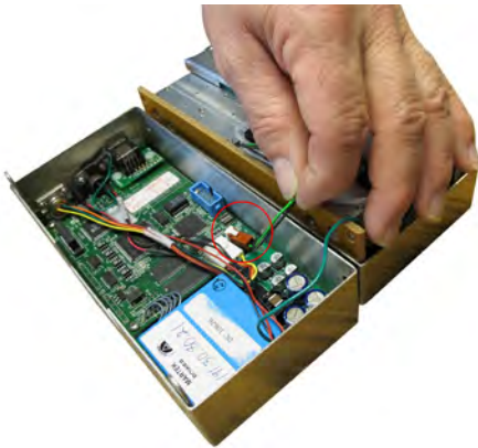
FIGURE 6.16: DISCONNECT THE QUICK ZERO SOLENOID
