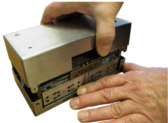
FIGURE 6.14: SEPARATE THE CASE HALVE SCREWS
