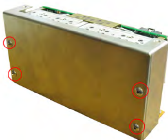
FIGURE 6.17: REMOVE THE CORE
