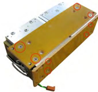
FIGURE 6.18: REMOVE THE INSULATORS
