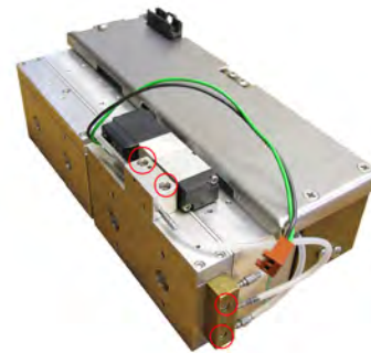
FIGURE 6.19: REMOVE THE MANIFOLD
