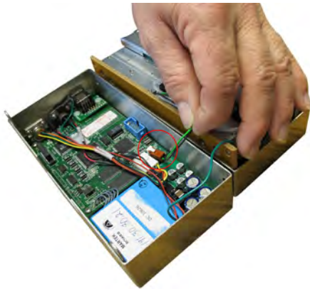
FIGURE 6.16: DISCONNECT THE QUICK ZERO SOLENOID
