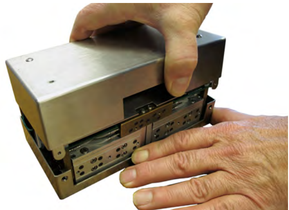
FIGURE 6.14: SEPARATE THE CASE HALVE SCREWS
