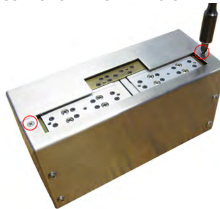
FIGURE 6.13: REMOVE THE CASE HALVE SCREWS
