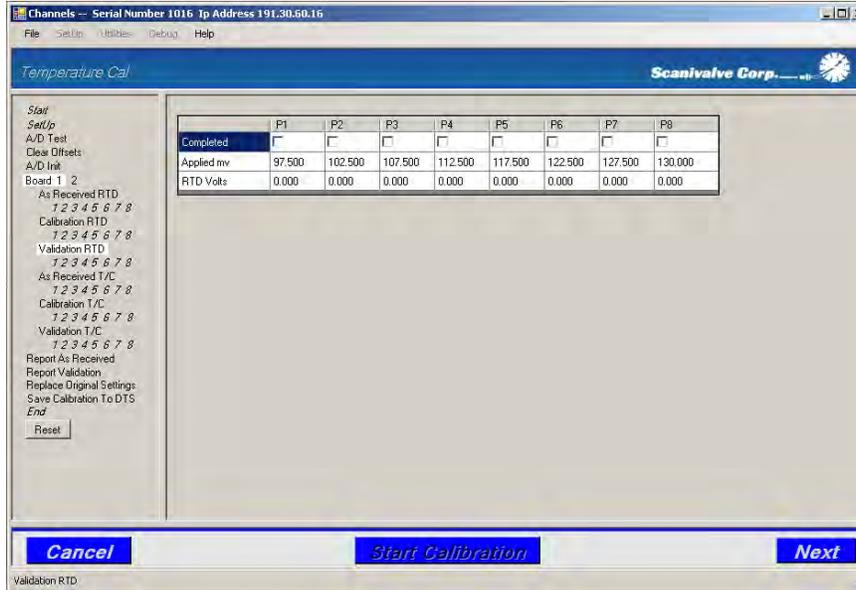
The next screen will prompt the user to input a known voltage using a voltage standard. This screen displays the voltage to be applied (**'Apply - - -:'**) as well as a reading of the currently applied voltage. Once the voltage has been applied and is stable, click **'Next.'**
