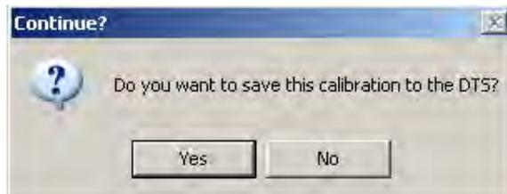
In order to restore the original calibration coefficients the DTS must be rebooted. After the 'No' button is pushed deciding not to save the new calibration coefficients, TempCal automatically reboots the DTS. A message window appears noting this. Pressing the 'OK' button is required to complete the test and restore the original calibration. As prompted in the message window, it may take several minutes for the DTS to reboot allowing a connection to be established again.
