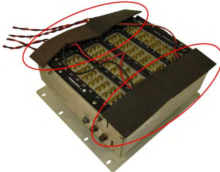
8) Install the cover. After powering the unit up, let the DTS thermally stabilize for a minimum of 3 hours before beginning the calibration.
