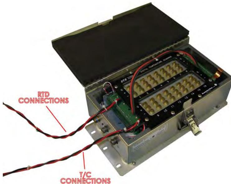
For each calibration harness, there is one RTD connection and one T/C connection. **The RTD connection for the voltage standard is labeled 'RTD.'** Connect the RTD connection, and click 'Next.'
