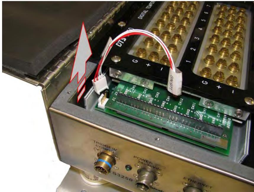
3) Install calibration harness connector #1
