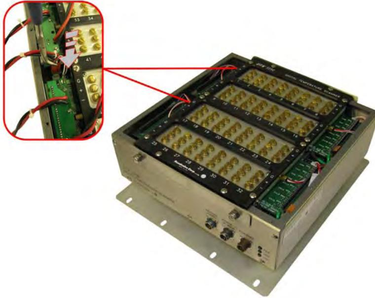
7) Place insulation over the exposed connectors
