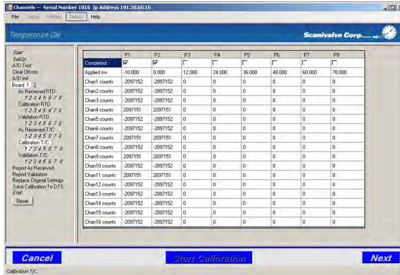
The next screen will prompt the user to input a known voltage using a voltage standard. This screen displays the point number and the voltage to be applied as well as a reading of the currently applied voltage (in raw counts). Once the voltage has been applied and is stable, click 'Next.'
