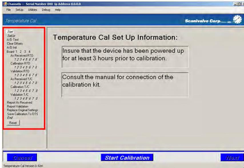
Alternately, the test controls can be configured by selecting on of the pre-configured test setups found in the **Setup Menu**. See the section devoted to the **Setup Menu** in the **Getting Started** section of this manual.
