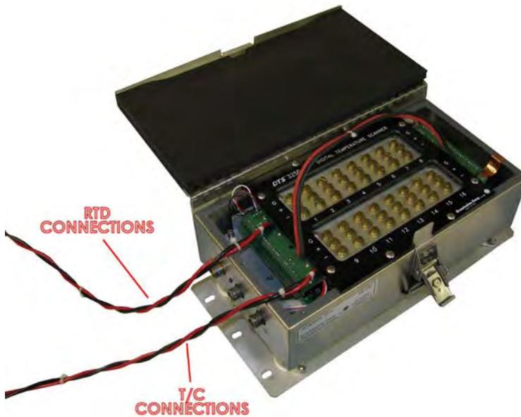
For each calibration harness, there is one RTD connection and one T/C connection. **The T/C connection for the voltage standard is labeled 'T/C.'** Connect the T/C connection to the voltage standard and click 'Next.'
