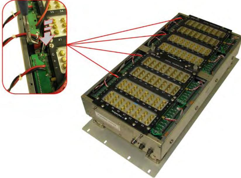
7) Place insulation over the exposed connectors
