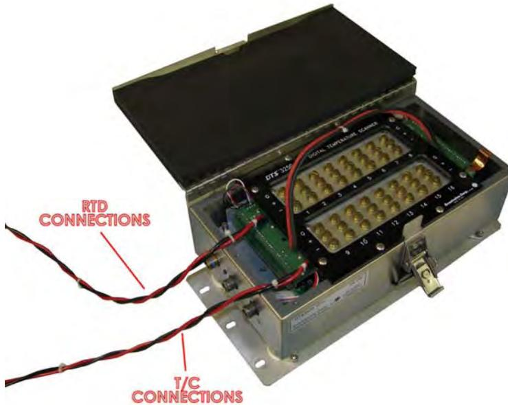
For each calibration harness, there is one RTD connection and one T/C connection. **The RTD connection for the voltage standard is labeled 'RTD.'** Connect the RTD connection to the voltage standard and click 'Next.'
