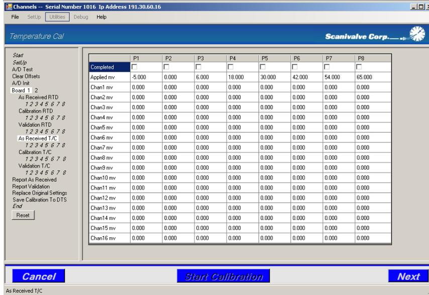
The next screen will prompt the user to input a known voltage using a voltage standard. This screen displays the point number and the voltage to be applied as well as a reading of the currently applied voltage. Once the voltage has been applied and is stable, click **'Next.'**
