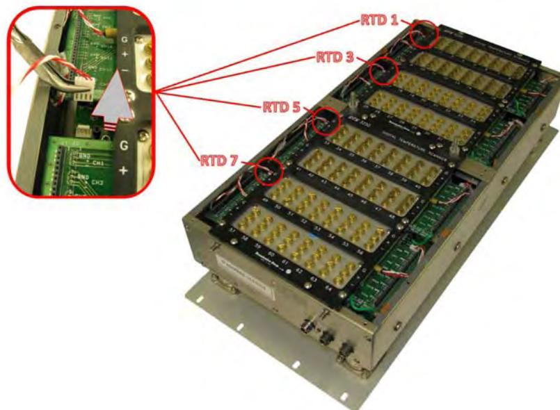
4) Install calibration harness connector #1 (4x)
