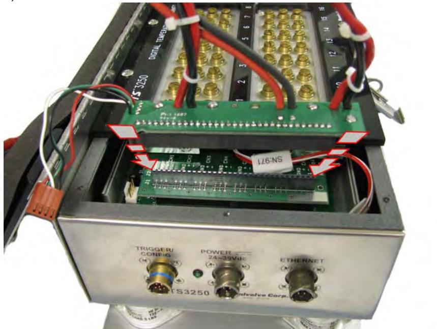
4) Install calibration harness connector #2
