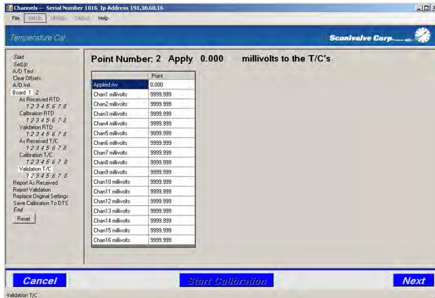
TempCal will return to the front screen and indicate that the point has been validated with a check mark in the box below the point. Continue through each point until all points have been validated.
