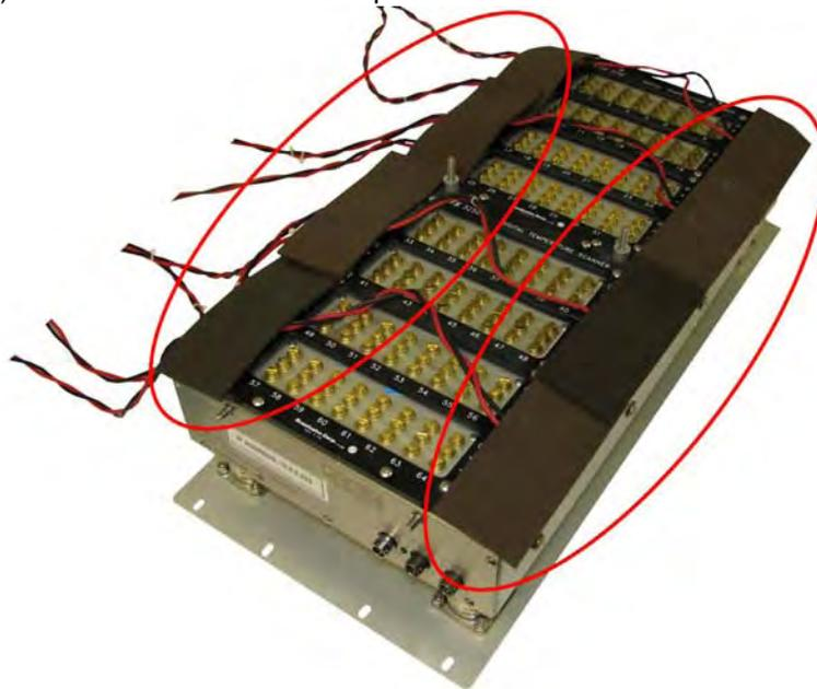
8) Install the cover. After powering the unit up, let the DTS thermally stabilize for a minimum of 3 hours before beginning the calibration.
