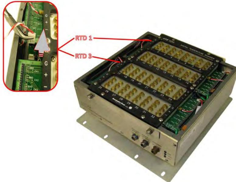
4) Install calibration harness connector #1 (2x)
