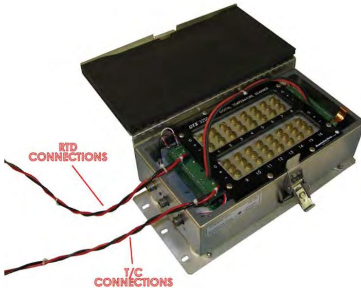
For each calibration harness, there is one RTD connection and one T/C connection. **The T/C connection for the voltage standard is labeled 'T/C.'** Connect the T/C connection, and click 'Next.'
