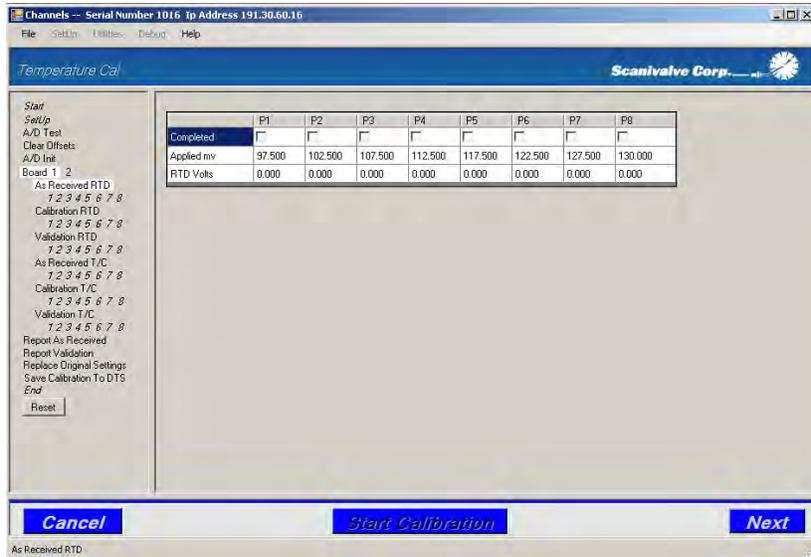
The next screen will prompt the user to input a known voltage using a voltage standard. This screen displays the voltage to be applied ('Apply ---: ') as well as a reading of the currently applied voltage. Once the voltage has been applied and is stable, click 'Next.'
