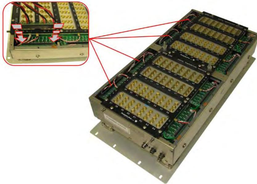
5) Install calibration harness connector #2 (4x)
