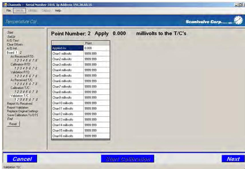
TempCal will return to the front screen and indicate that the point has been validated with a check mark in the box below the point. Continue through each point until all points have been validated.
