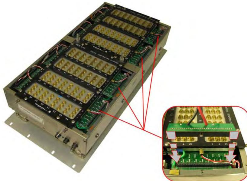
6) Install calibration harness connector #3 (Where the RTD was disconnected. 4x)
