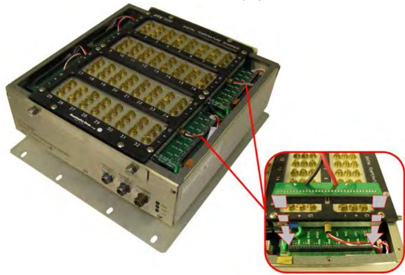
6) Install calibration harness connector #3 (Where the RTD was disconnected. 2x)
