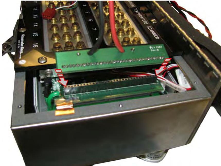
5) Install calibration harness connector #3 (Where the RTD was disconnected.)
