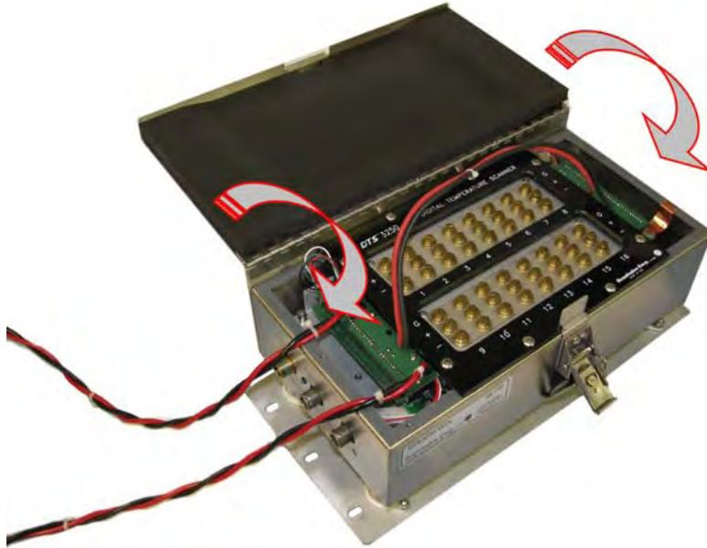
7) After powering the unit up, let the DTS thermally stabilize for a minimum of 3 hours before beginning the calibration.
