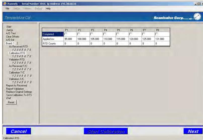
The next screen will prompt the user to input a known voltage using a voltage standard. This screen displays the voltage to be applied ('Apply - - - -:') as well as a reading of the currently applied voltage (displayed in raw counts). Once the voltage has been applied and is stable, click 'Next.'
