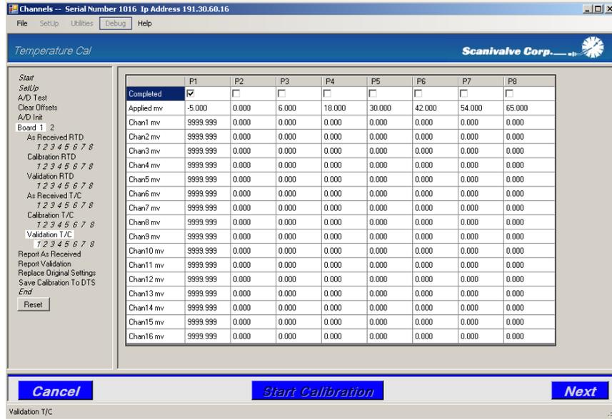
The next screen will prompt the user to input a known voltage using a voltage standard. This screen displays the point number and the voltage to be applied as well as a reading of the currently applied voltage. Once the voltage has been applied and is stable, click 'Next.'
