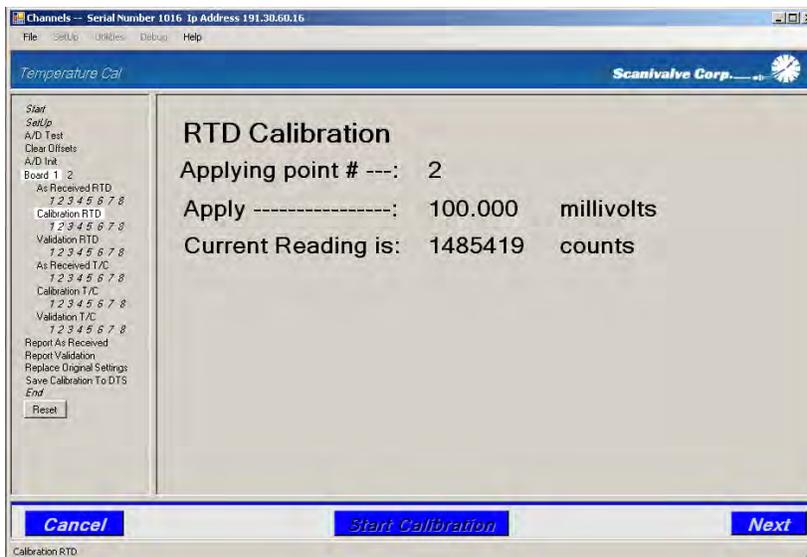
TempCal will return to the front screen and indicate that the point has been calibrated with a check mark in the box below the point. Continue through each point until all points have been calibrated.
